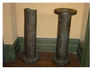
In the 18<sup>th</sup> Century, the Kings Vessels were equipped with pumps which allowed the removal of water from the bottom of the ship (the bilge). Each pump was approx. 10 metres in height and composed of three parts: 2 parts constructed of wood either end of a cental bronze cylinder.
